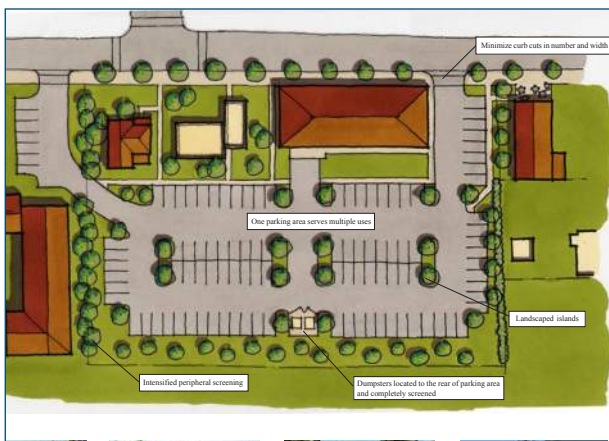
The Old Coppel Master Plan recommends creating parking areas that serve multiple uses, thus making it easier to create a “building enclosure” along streets as depicted above.
