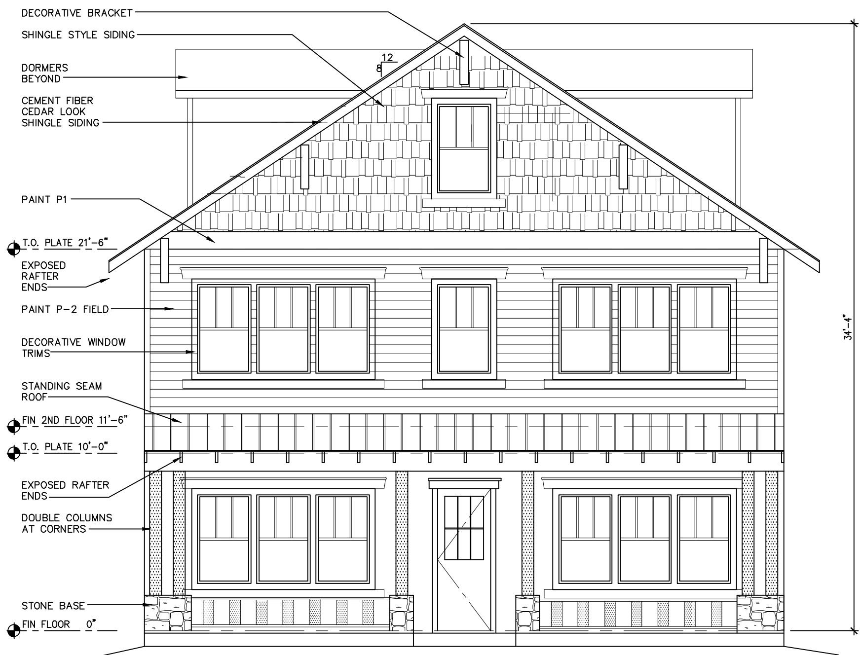
BLDG 6 EAST ELEVATION
