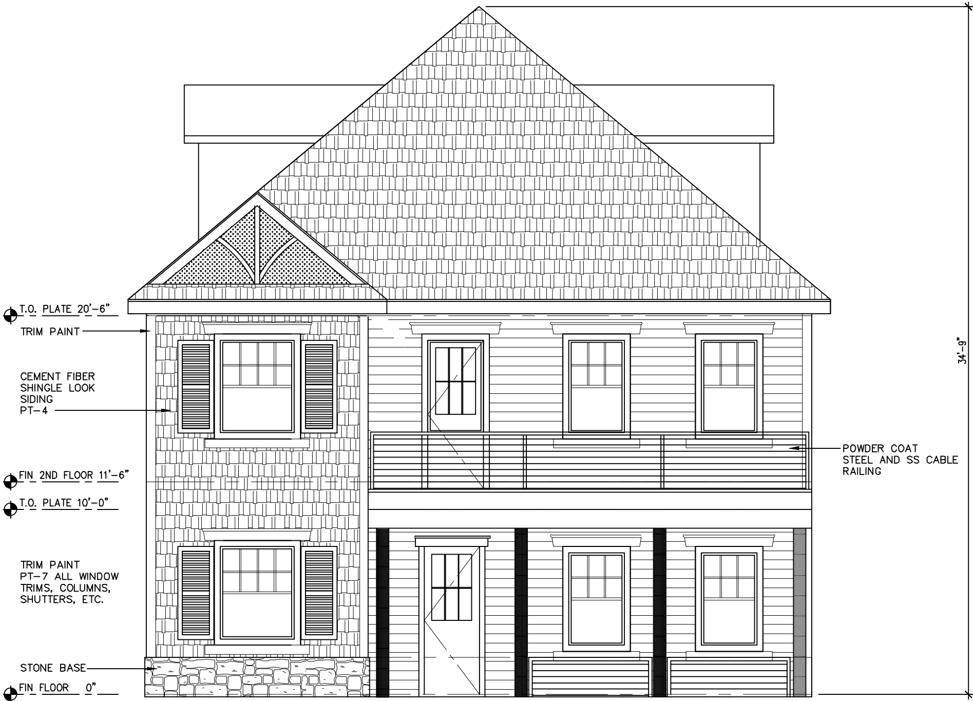
BLDG 4 EAST ELEVATION
