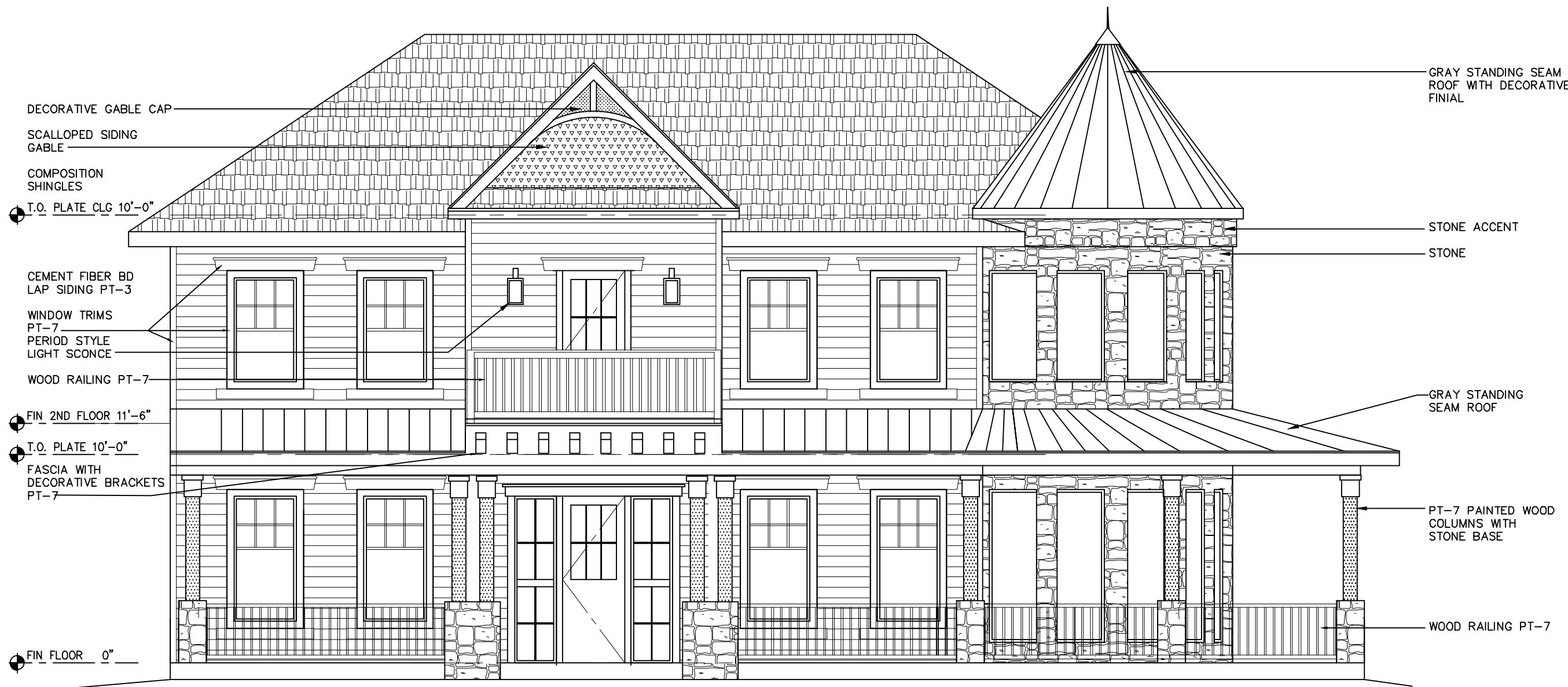
BLDG 3 EAST ELEVATION
