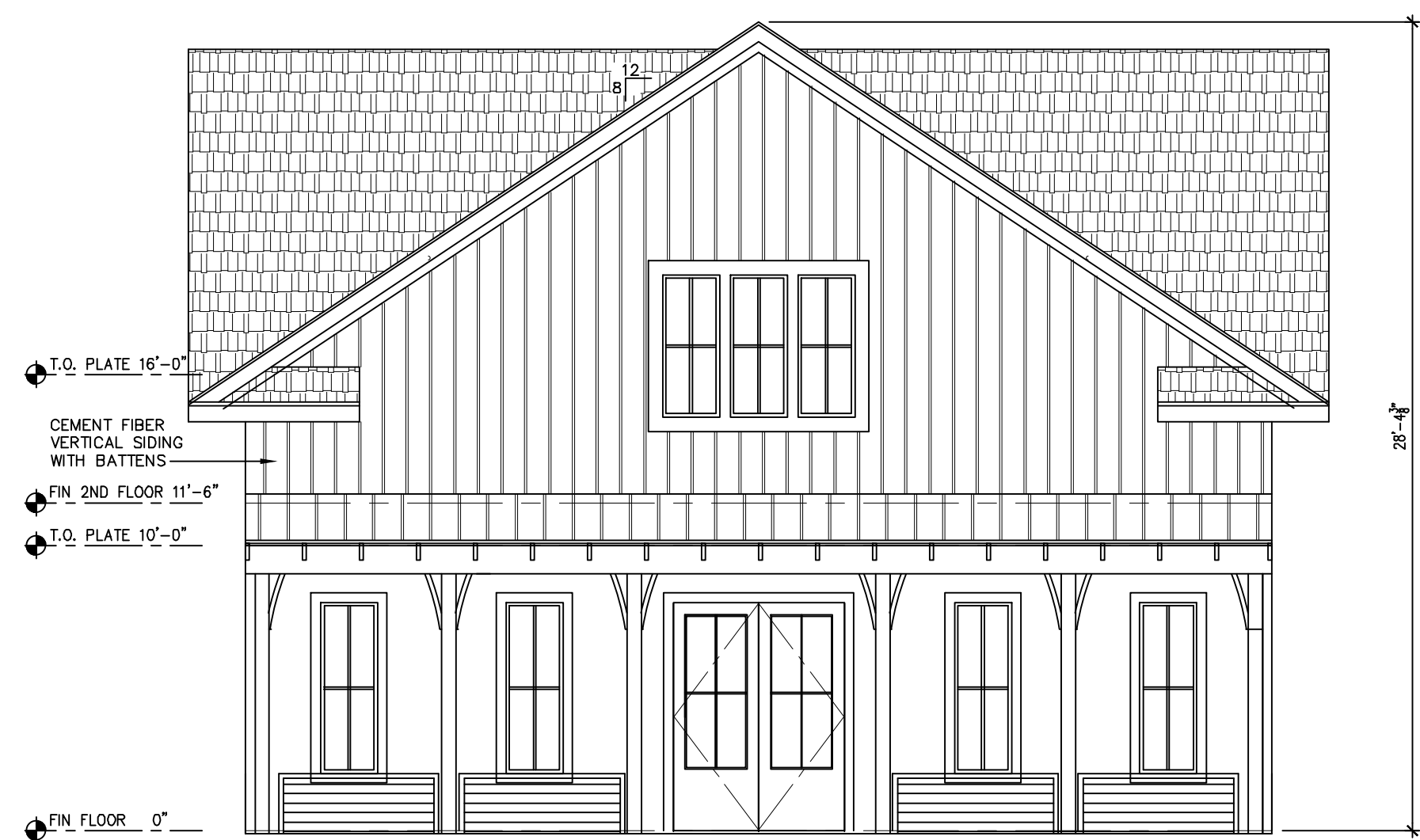
BLDG 5 EAST ELEVATION
