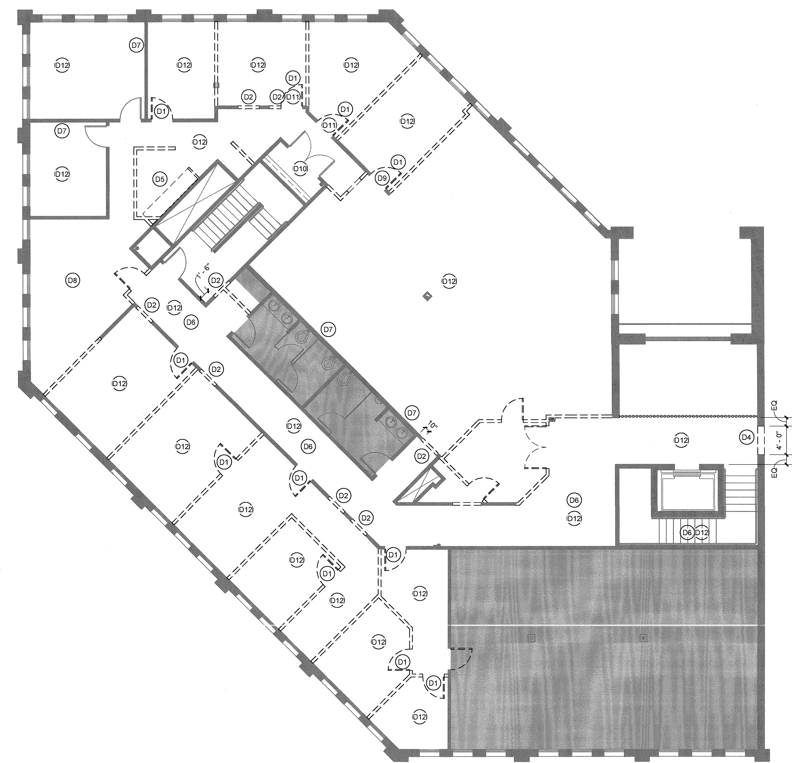
01 DEMOLITION PLAN - LEVEL 2 1/8" = 1'-0"
