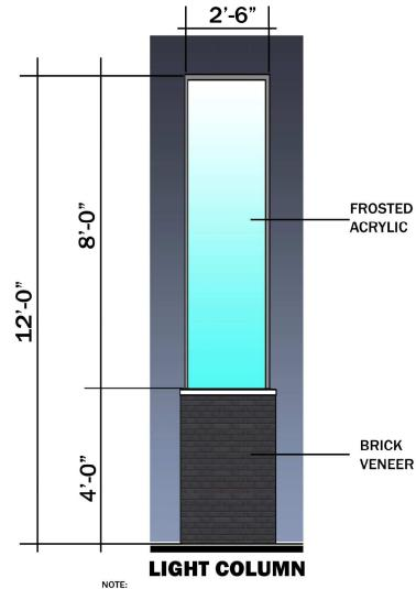
NOTE: ESTIMATED DIMENSIONS, FINAL DIMENSION TO BE ESTABLISHED DURING DETAILING
