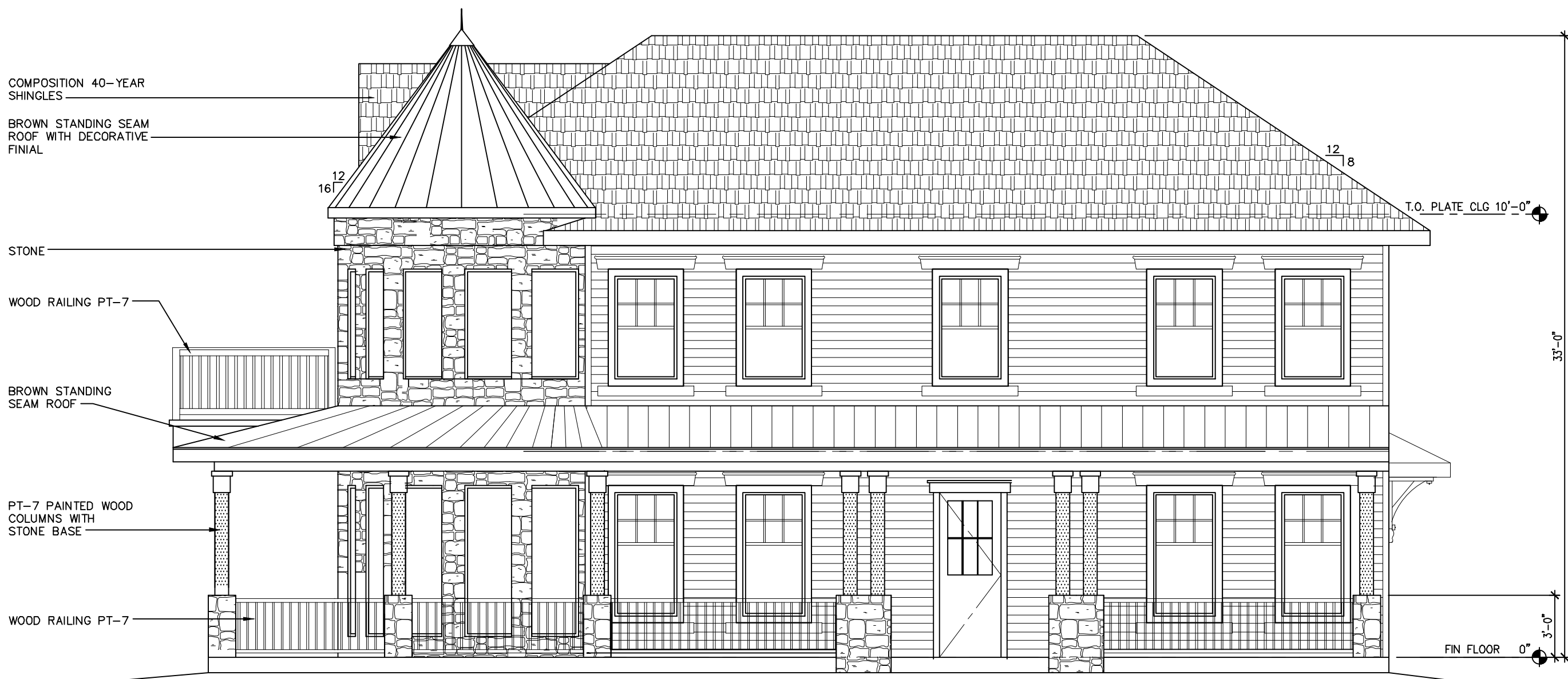
BLDG 3 NORTH ELEVATION
