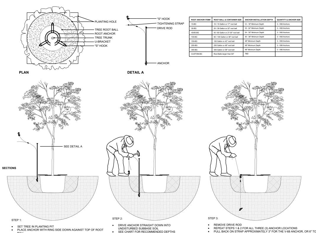
• CENTER ROOT ANCHOR'S INNER RING(S) AROUND TRUNK OF TREE ALIGN DRIVE ROD AS CLOSE AS POSSIBLE TO OUTSIDE EDGE OF
