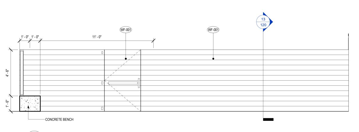
13 EXTERIOR COURTYARD ELEVATION SCALE: 3/8" = 1'-0"
